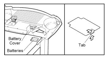
are touching the springs in the battery compartment. Close the battery cover, push up on the battery cover tab, and then push the tab forward as shown in the inset drawing. Make sure that the tab locks into place.
